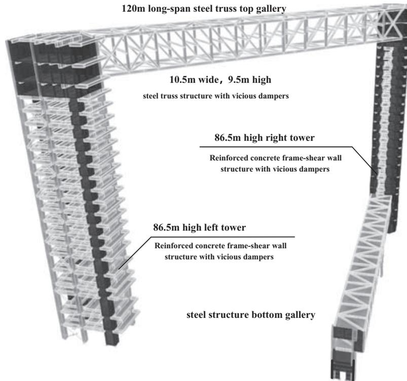
Figure 2. Three-dimensional schematic diagram of the connected tall building structure
