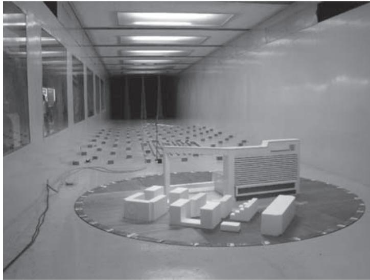
Figure 4. Wind tunnel test model
