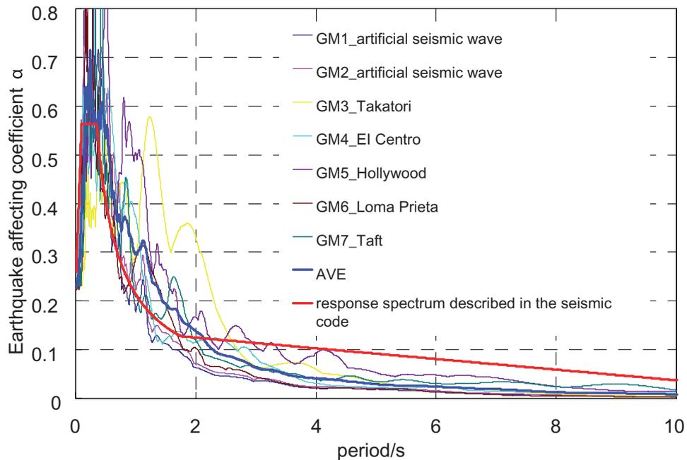
Figure 3. Comparison of response spectrum from the seismic code and seismic waves
