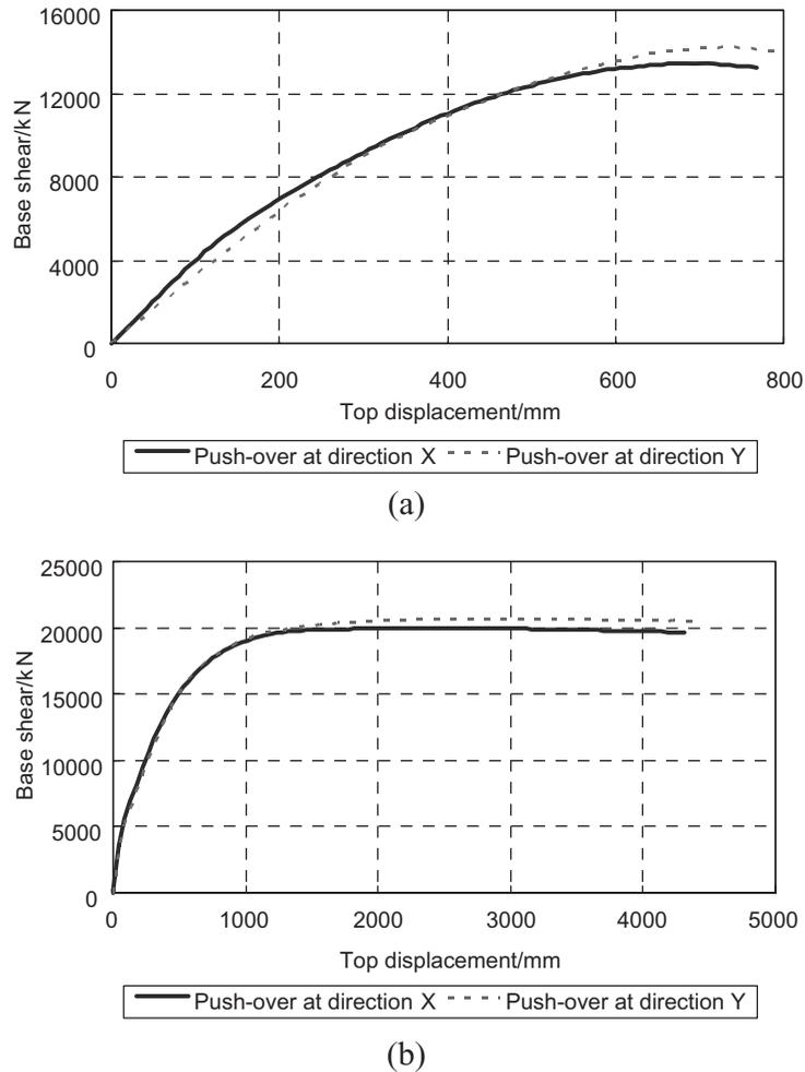
Figure 8. Top displacement–base shear curve: (a) the left tower and (b) the right tower
